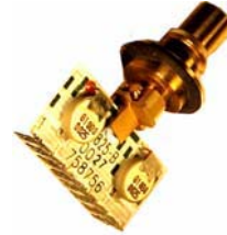
Gripper nozzle with a hybrid circuit
